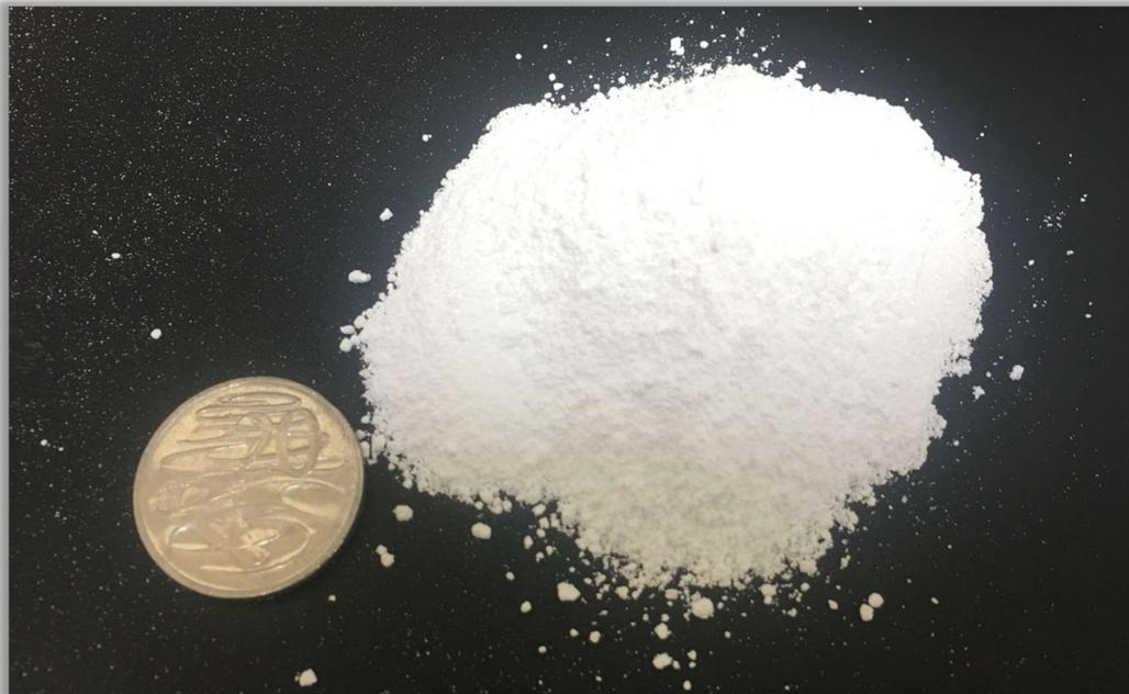
Sample of High Purity Alumina generated from the HPA First process
